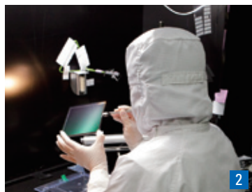
1 Some of the latest photomask products can cost several hundred million yen per set 2 Pellicles are manufactured and checked in a clean-room environment
