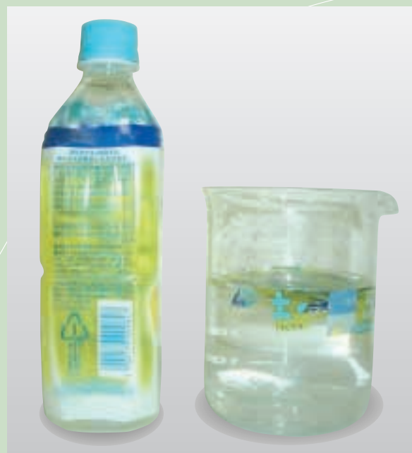
Label of polyolefin resin (above) Sinking PET resin and floating polyolefin resin in water (upper right) Photo 1
