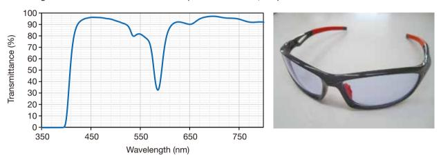
Light Transmittance of NeoContrast<sup>TM</sup> is shown in the left diagram and an example of NeoContrast<sup>TM</sup> lenses (sports glasses type) in the right photograph.
