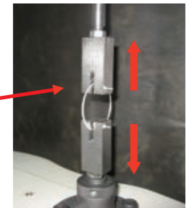
Test for tensile strength of lens materials
