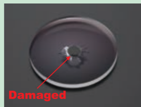
Middle-Index & Acrylic lenses were broken ADC lens had cracks
